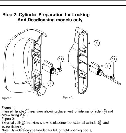
1 Remove screw (14) and extract cylinder if necessary.
