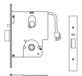
Door type: Metal or wood Backset: 60mm standard. 70mm, 89mm and 127mm available Fire rated: 4 hours - refer fire door manufacturer for approval Door thickness: 32mm to 50mm
